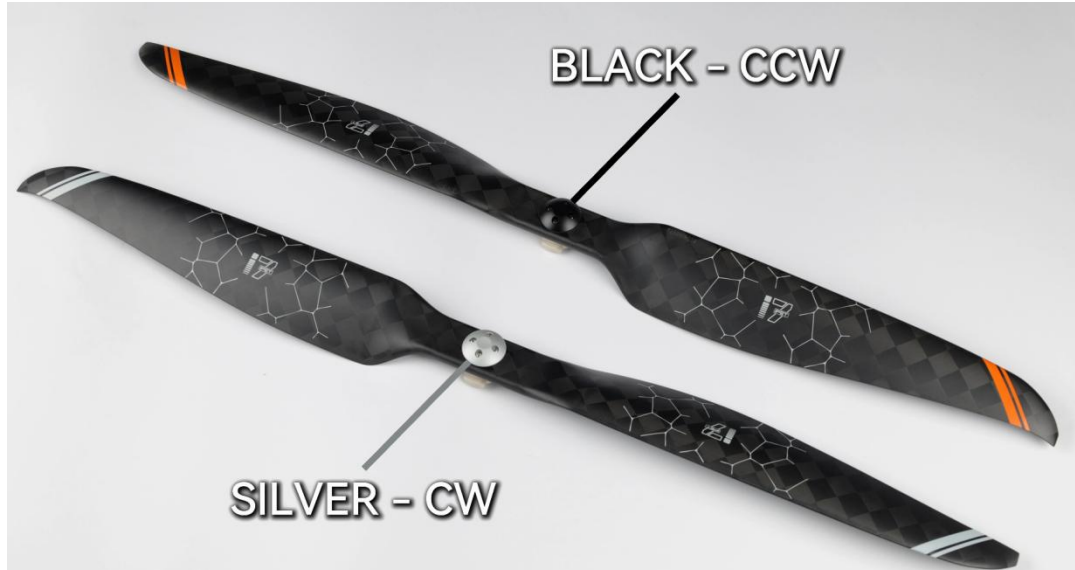
Step 1: Distinguishing between CCW and CW Propellers
