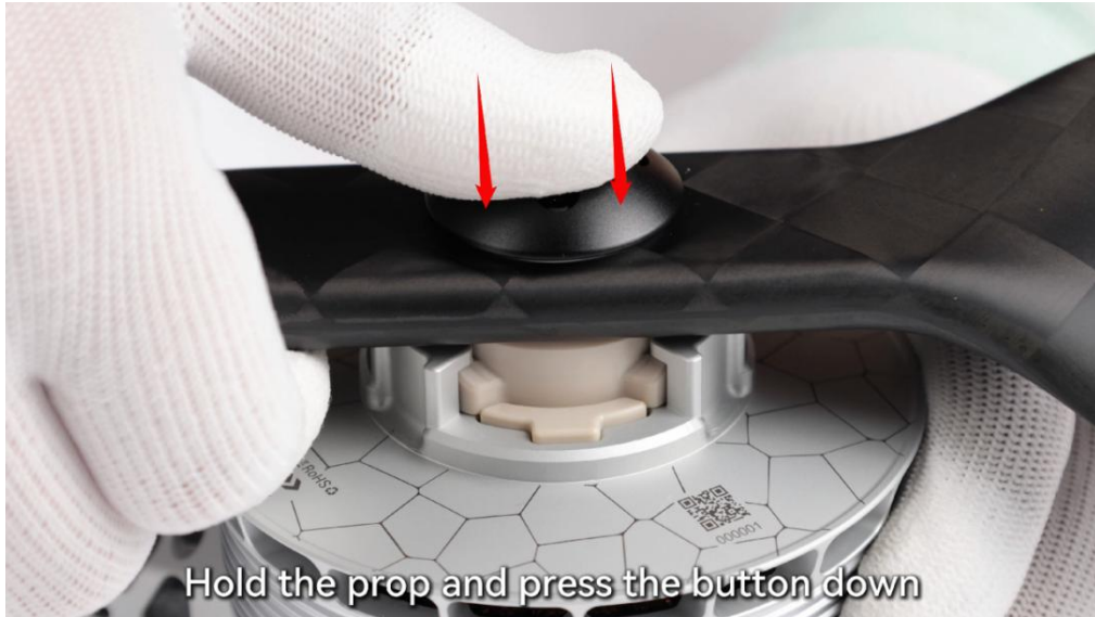
Step 1: Hold the propeller and press the button downwards
