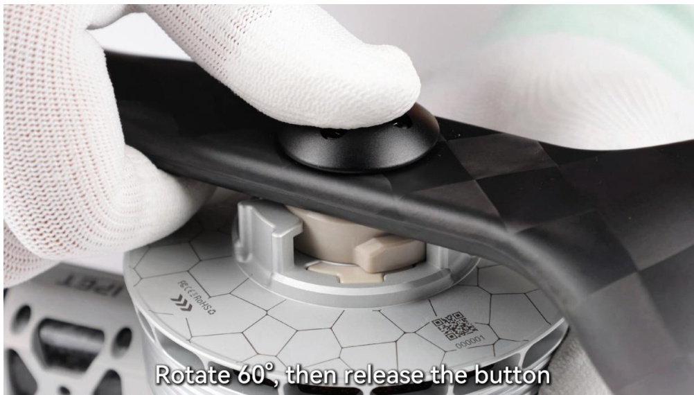
Step 2: Rotate 60° while pressing, then release the button to remove the propeller
